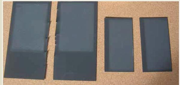
**Above:** After 2000 hours of UV testing the New Zealand product showed no evidence of degradation compared with the imported product (below) tested under the same conditions. Photographs used with the permission of NZMRM.
